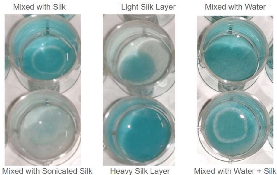
Figure 9. Paper tests of various formulations were stored at room temperature for approximately 3 months. Formulations included water-based X-Gluc solution only, silk fibroin mixed with X-Gluc, silk fibroin layered over X-Gluc, and silk fibroin-based gel with X-Gluc. Pure enzyme was then added to the tests, and images were taken for up to 90 minutes (pictured) to compare intensity and time required for the reaction.
