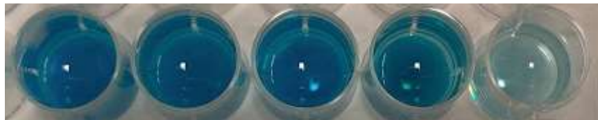
Figure 4. From left to right, decreasing concentrations ( 10^8 , 10^7 , 10^6 , 10^5 , and 10^4 CFU) of E. coli in reaction with X-Gluc.
